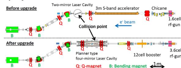
Figure 1: The beamline of the LUCX accelerator before/after upgrade.
