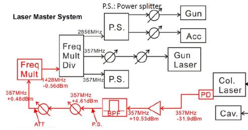
Figure 5: Diagram of the laser master system.
