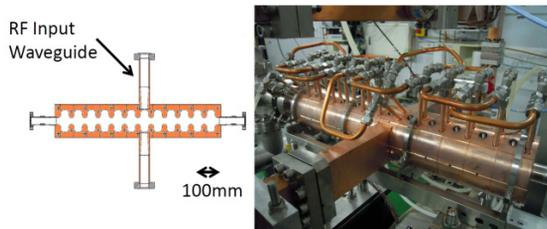
Figure 3: The cut view and the picture of the 12cell booster.
