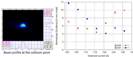
Figure 7: The left picture is the beam profile at the collision point. The right graph shows the result of emittance measurement.
