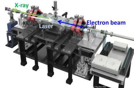
Figure 4: Drawing of the 4-mirror planar optical cavity.
